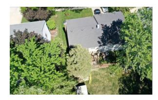
Photo showing potential obstructions. This photo attempts to show the impact of the two large trees to the south of the array location. This shading can influence REC quantity and incentive amounts and could justify alternative design methods.
