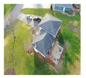
Photo showing proposed array location for a single-family residence. This one aerial photo would satisfy requirements when multiple arrays are placed on the different directional facing pitches of the roof. However, photos taken from 6' above the roof will not capture all the proposed arrays, in which case multiple photos will need to be presented.
