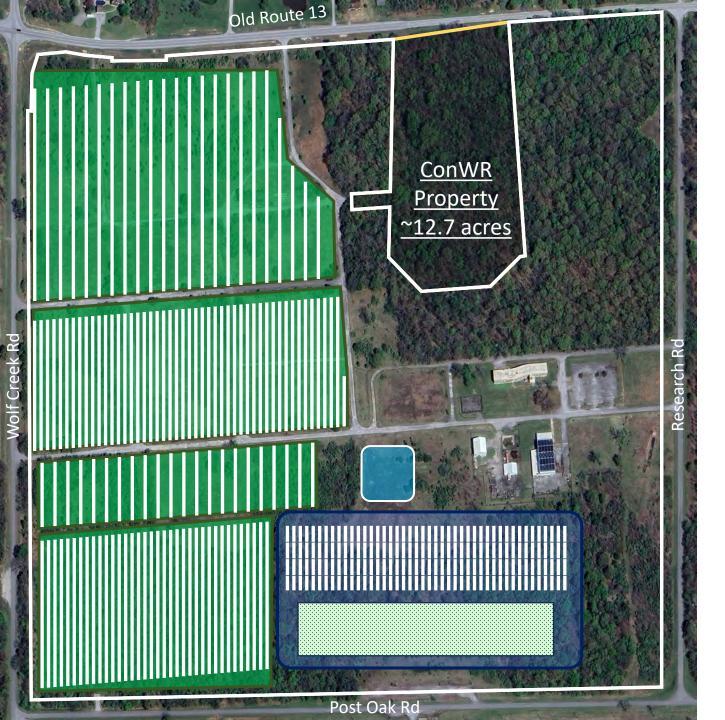
SI-Spear will produce  $^{\sim}10MW_p$  (AC) (12.3 MW DC) low-cost power.
